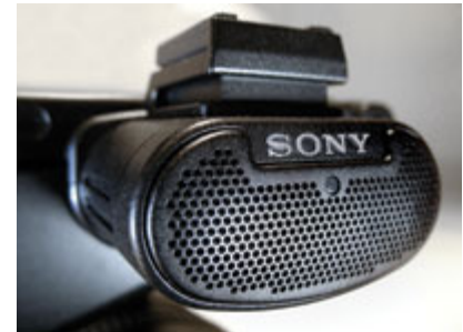
The Z5 brings back the built-in stereo mic that is missing from the Z7.
