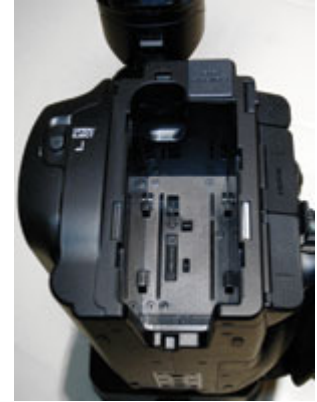
The battery well of HVR-Z5U is deeply recessed to fully enclose large NP-F970 InfoLithium battery so that the HVR-MRC1 Memory Recording Unit using CompactFlash can attach flush to rear.
